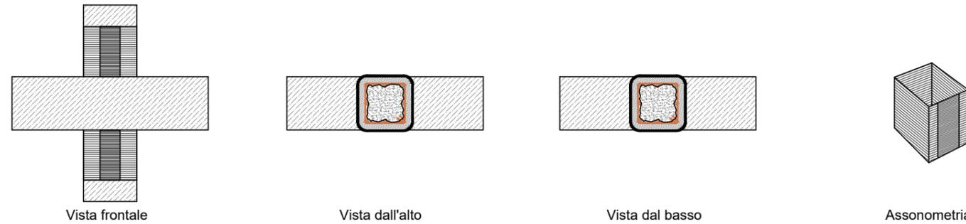
INCREMENTO DELLA RESISTENZA A TAGLIO DELLE ESTREMITÀ DELLE TRAVI
