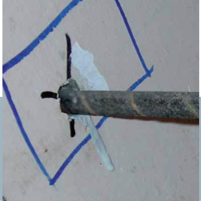
**Pultruded carbon bar with improved adhesion for FRCM structural strengthening system**
